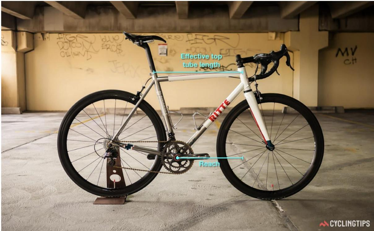
An important, and often overlooked, measurement is the top tube length. You may have long legs and a short torso (or vice versa), which means that you'll be leaning into the handlebars too much, causing unwanted tension in your neck, shoulders, and lower back.
