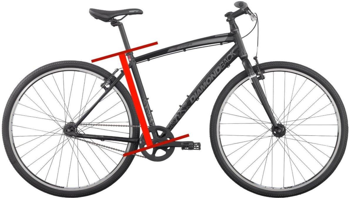
Although not very accurate bikes are still measured mainly by the bike frame size, which is the length of the seat tube. This is the vertical tube beneath the seat which runs down to the point where the crankshafts and pedals are attached to the bike frame. The length is measured from the top point where the seat is attached, to the bottom bracket where the crank is bolted to the frame.
