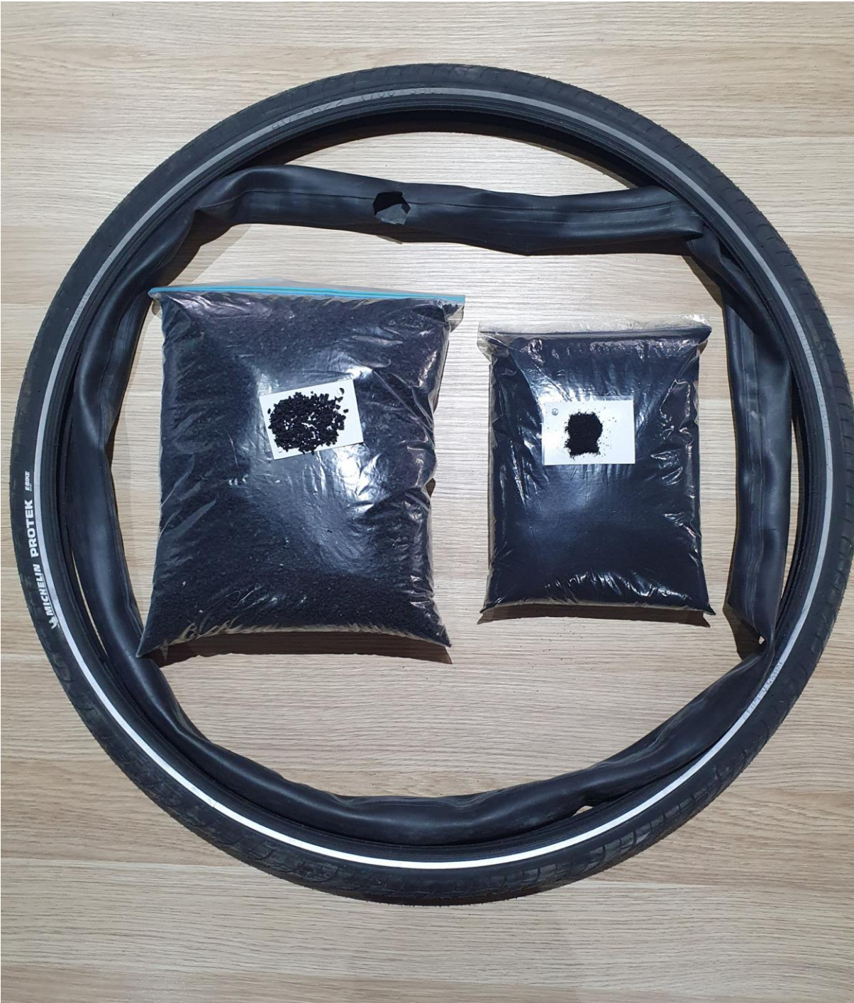
Tyres & tubes turned into granules (L) for playgrounds & 30 mesh (R) for roads
